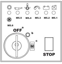
M5.1 (yellow) Fuel reserve M5.2 (yellow) Battery charge M5.3 (red) Overspe-M5.4 (red) High temperature M5.5 (red) Low oil pressure M5.6 (green) Protection unit on
