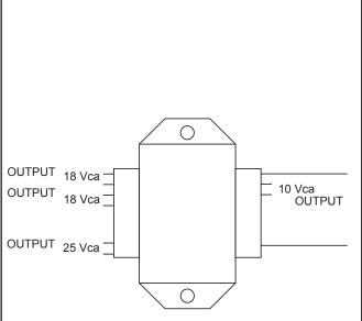
Check the transformer in this way:
