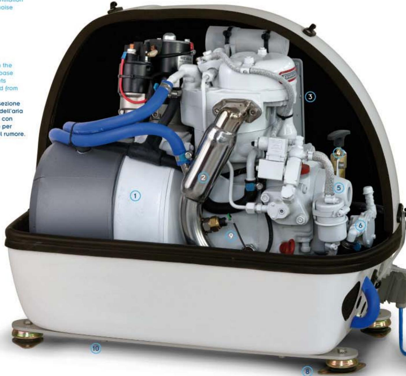
9 Engine oil cooled by a sump mounted stainless steel heat exchanger and combustion intake air cooled by watercooled air intercooler, ensuring the power output of the generator is not affected by high ambient air temperatures.
