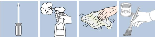
Procedure**3.1 Remove the gasket (3a)****3.2 Remove the components (3b, 3c, 3d)****3.3 Clean and lubricate the gasket housing and replace it with a spare part****3.4 Reassemble the components (3a, 3b, 3c, 3d)**
