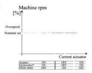
If the running speed of the engine reaches the **OVERSPEED** set point, while the system is in a running state, the S2007 will stop outputting a signal to the actuator for a zero fuel command and will no longer attempt to control the engine.
