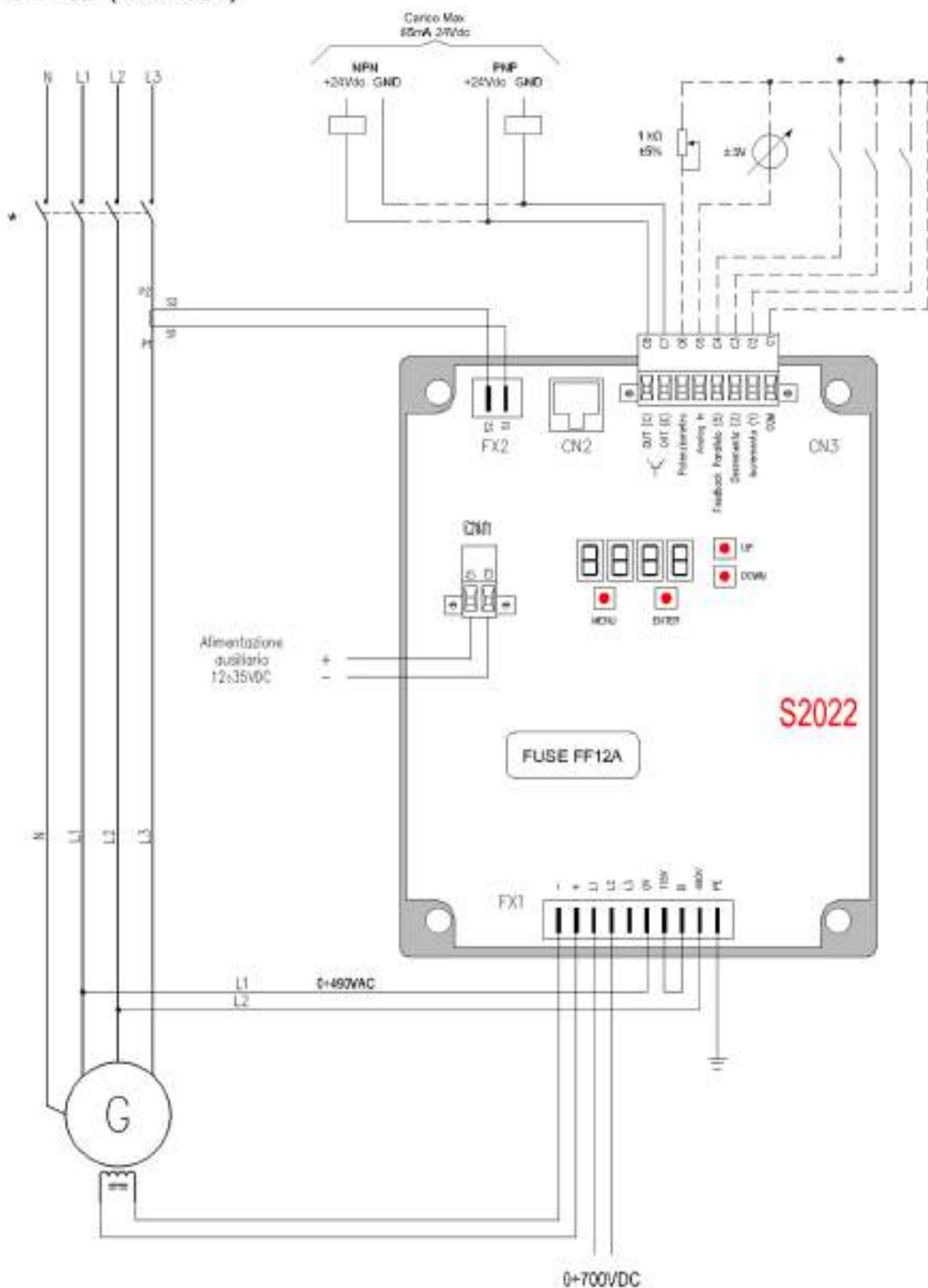
Connection with power source from auxiliary winding DC (MAX 440VAC) and voltage reference directly from riser (MAX 490 V).
