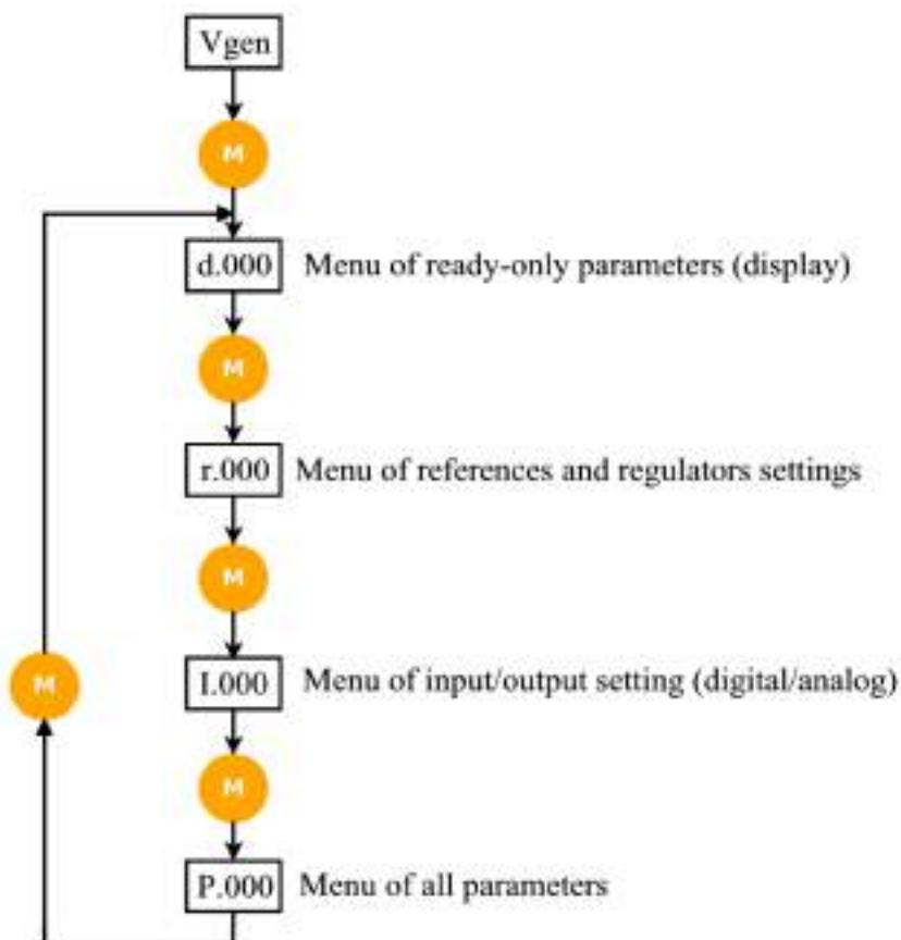
**Example: how to change a Rated voltage generator reference**
