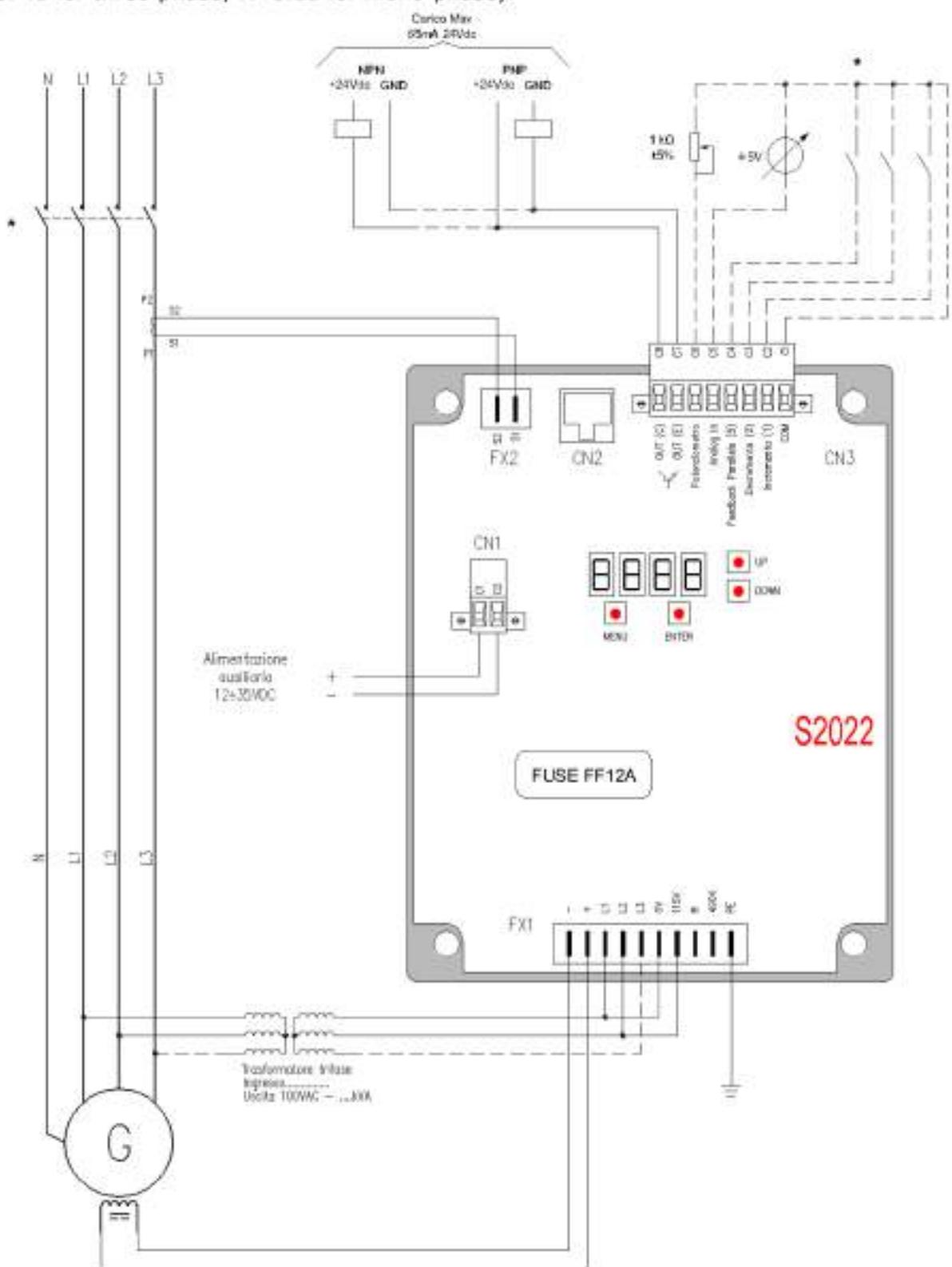
Connection with power source from PMG (mono or three phase Max 440V) and reference voltage direct from riser (MAX 490V).
