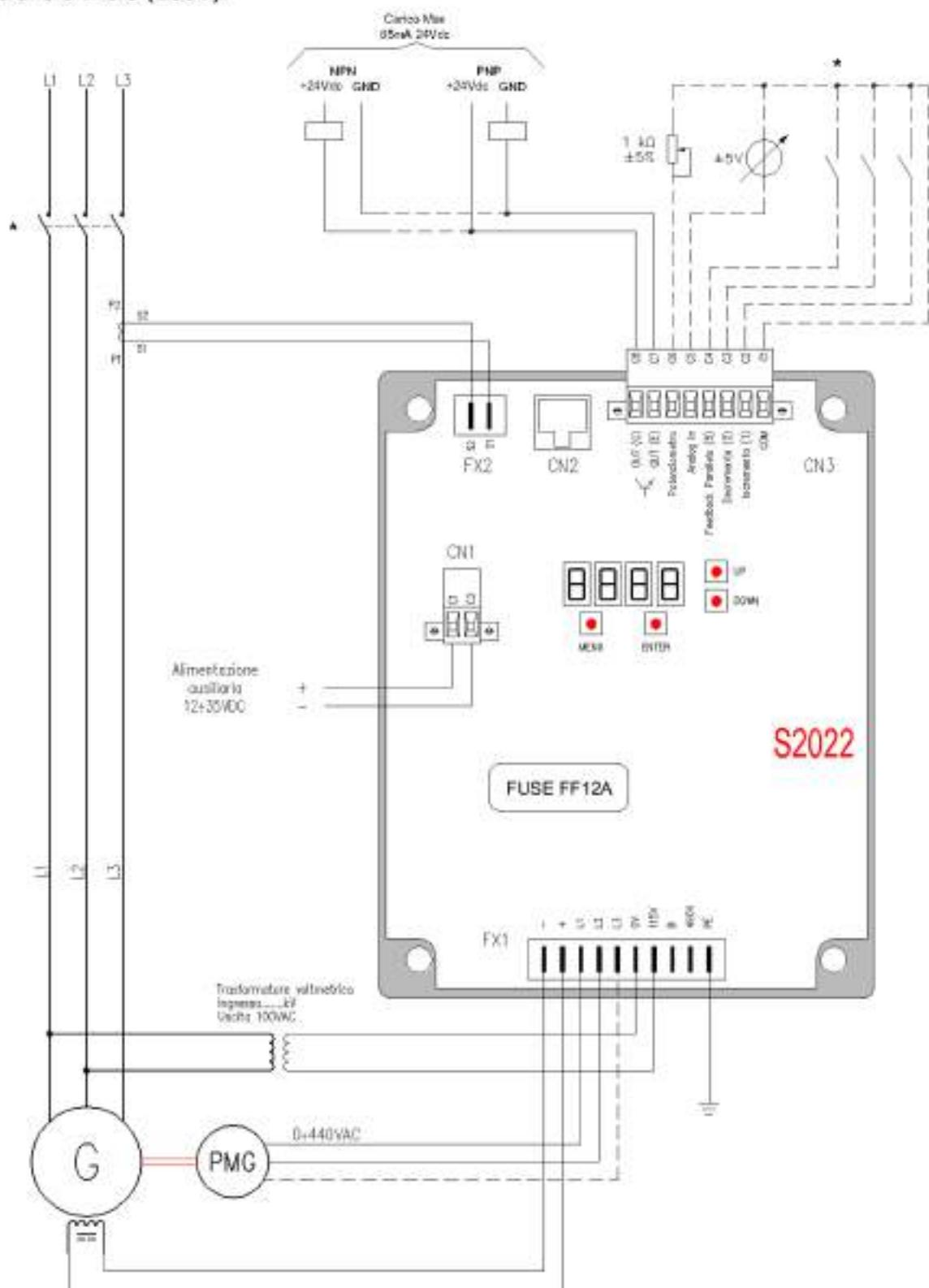
Connection with power source from DC auxiliary (MAX 700V) and reference voltage from voltage transformers (100V).
