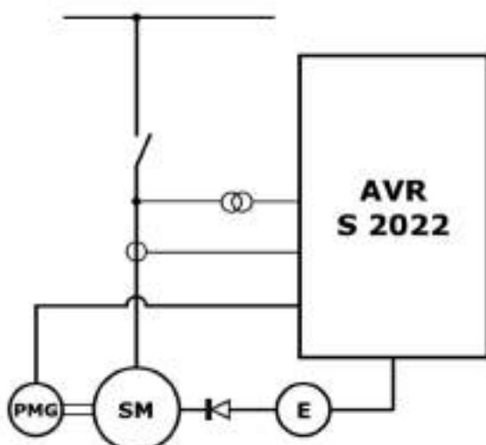
Replacement of voltage regulators for generators with direct-current excitation machines.
