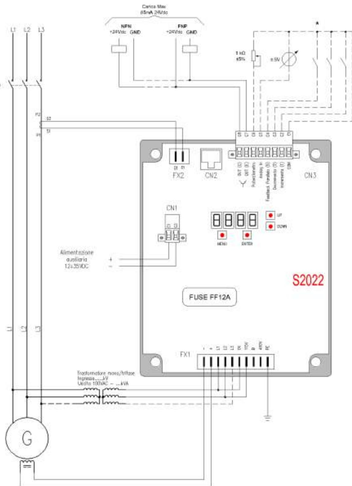
Connection with power source from PMG (Max 440V) and reference voltage from voltage transformers (100V).
