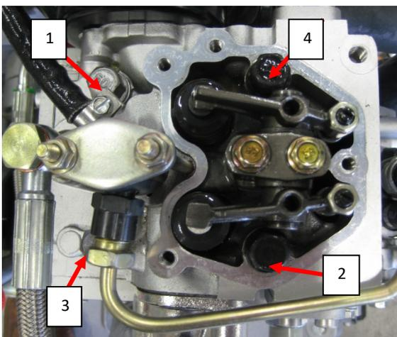
Figure 9: Cylinder head bolts
