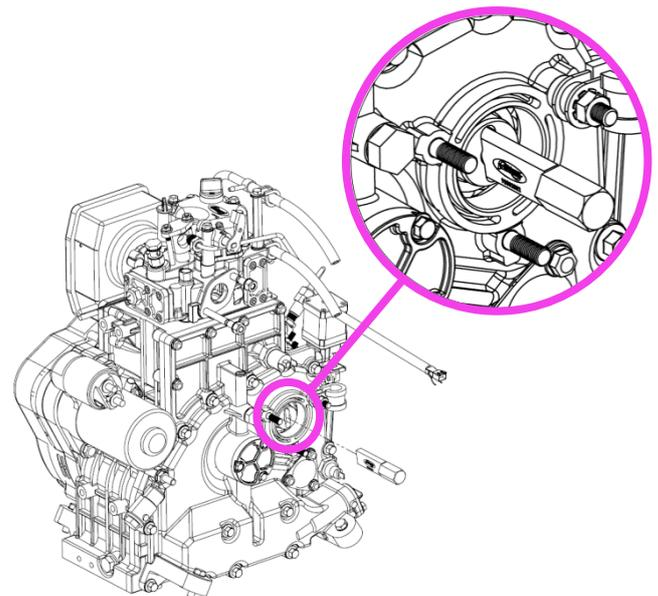
Figure 10: Turning tool to move to Top Dead Center position
